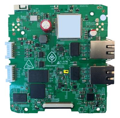
MANTARAY-enabled charge points can be connected together over Ethernet to provide load balancing between chargers. Dynamic load balancing with energy loads and sources is also possible. Multiple communication protocols can be supported.
